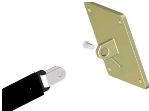
Image 3.10: Installing the energy absorber pin
