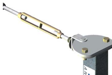
Image 3.13: Adjustment before installing the rope
