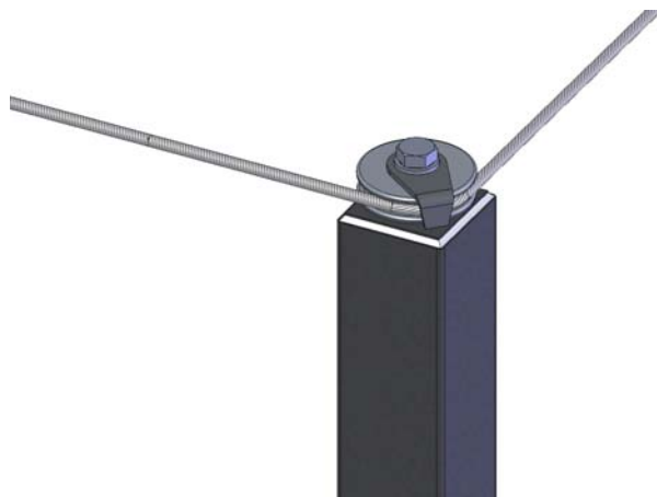
Image 3.8: Installing the curved section on the curved post
