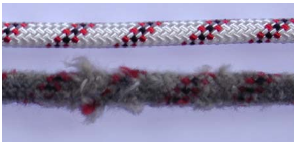
Fig. 2: Severe rope wear, wear with rope thickening
