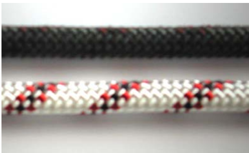
Fig.3: Blackening of the rope due to brake dust
